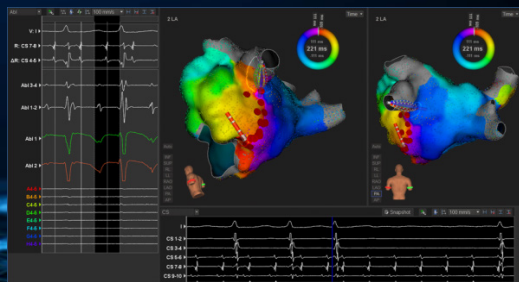
In a typical EP ablation procedure, the EP physician must be able to effectively guide the mapping catheter into the patient's heart (image on the left) and then manually navigate around the chambers to collect as many data-points of biopotential readings in order to create as accurate a heart-map (image on the right) as is possible within the time constraints of the procedure, in order to make prognostic decisions on where and how to make their ablation points to restore heart rhythm fidelity.
