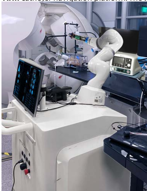
The Proteus™ Robotic Arm shown here with the Gripper attached, is undergoing final testing of its core navigation control functions in all of its operating modes at the NKC Animal Lab
