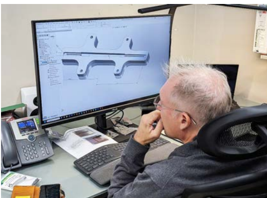
The image shows an engineer working on the design of the interface adapter that will allow the Huygens™ FCB to be integrated to the benchtop test board for in-house signal capture validation testing.
