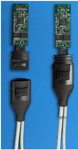
The image here shows the PM Phillips data communication assembly that will interface the Proteus™ Robotic Handle handle with the Ensite NavX.
