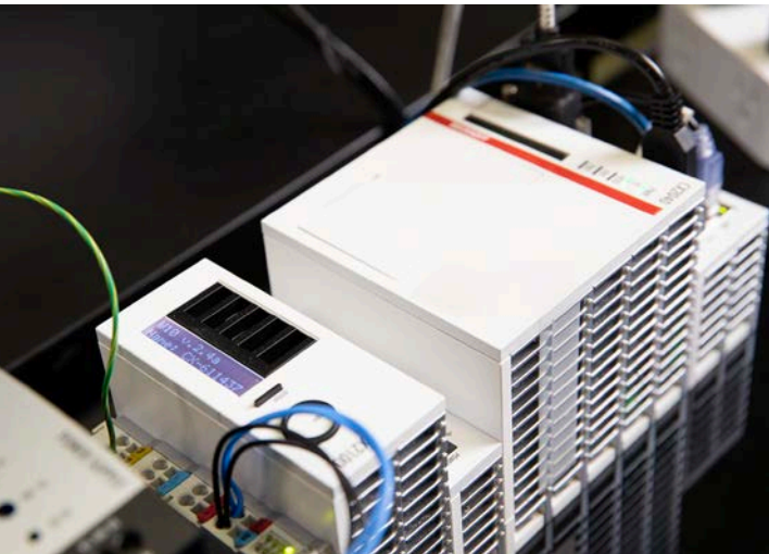
The NKC Programmable Logic Controller (PLC) operates much like a combination traffic cop and universal translator at the intersection of all data throughput in the NKC EP Operating Suite. The PLC takes all the incoming data streams, determines where it needs to go, converts the data into a language understood by the receiving device and then transmits that data to that device for processing.
