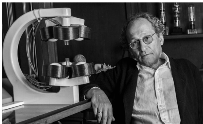
Inventor of the technology Josh Shachar with one of the first prototypes for the CGCI catheter guidance technology which was the progenitor for NKC's current achievements.
